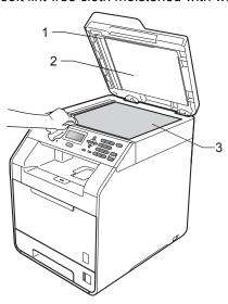
In the ADF unit, clean the white bar (1) and the scanner glass strip (2) underneath it with a soft lint-free cloth moistened with water.
